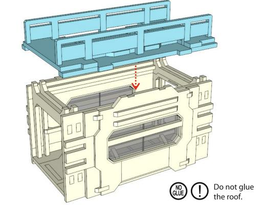
Hallway 240 construction process is the same as for Hallway 120, except step 2:
