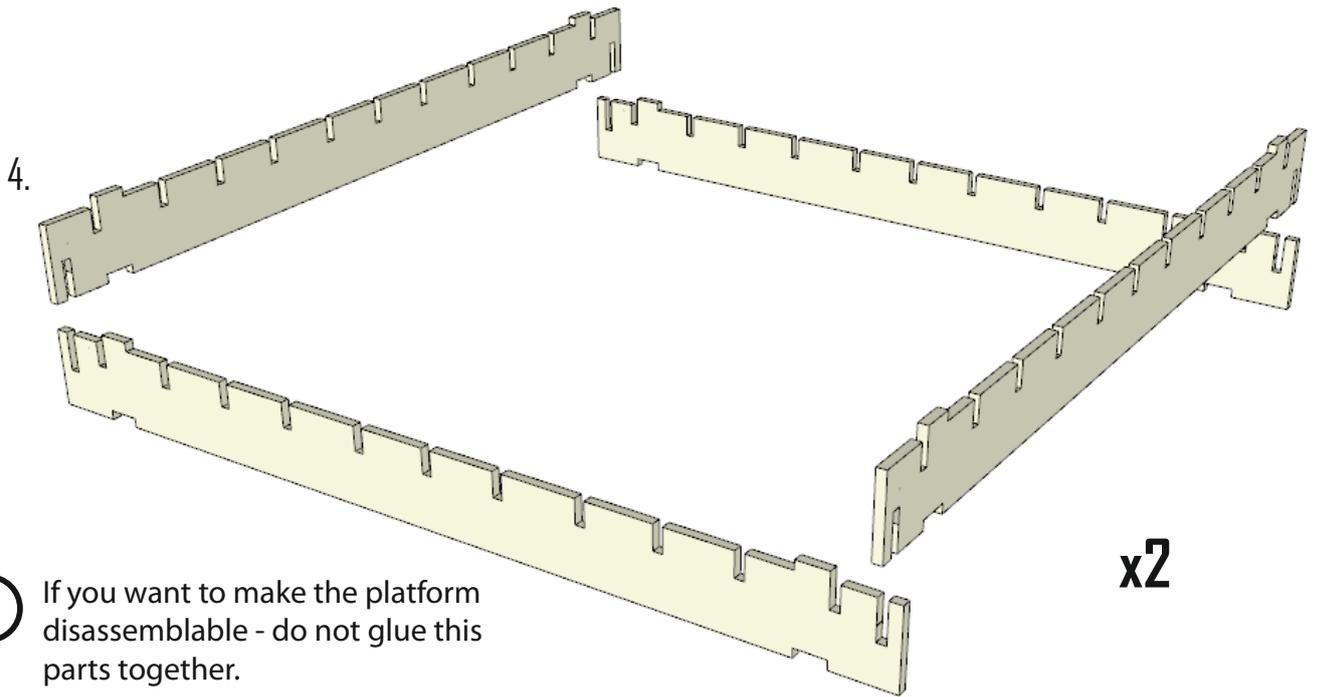
⚠ If you want to make the platform disassemblable - do not glue this parts together.
